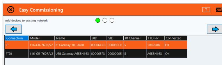
On the window that appears select the Gateway – network, in which the devices must join and click “**Next**” button.
