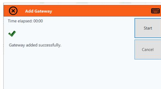
On the “116-GR-7600/V2” software “**Add IP Gateway**” window, you will see a confirmation message “**Gateway added successfully**”. Close the window and proceed into auto-detecting or easy-commissioning procedure.
