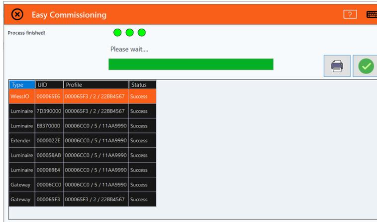
The system now is going through a procedure that sends unique commands to each selected wireless device to apply individual settings, so this may take a while. As a reference, for each Gateway and 100 wireless devices, it takes 20 minutes approximately. In the end, a full report of the procedure appears. You can print this report before exiting if there are failures, to review later.
